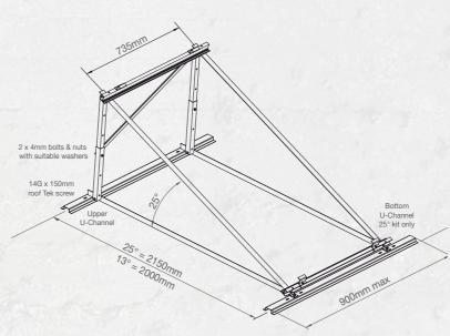
N.B. Collector size (1023 x 1941mm) is greater than frame size.
