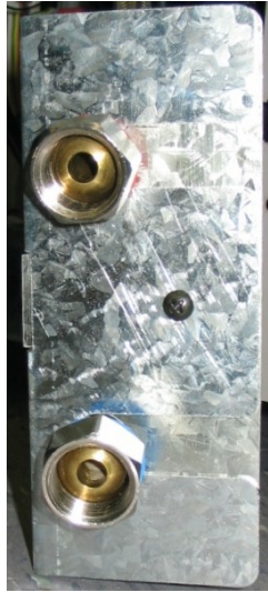
Step 8 assemble hose mount angle and hose clamp brackets
