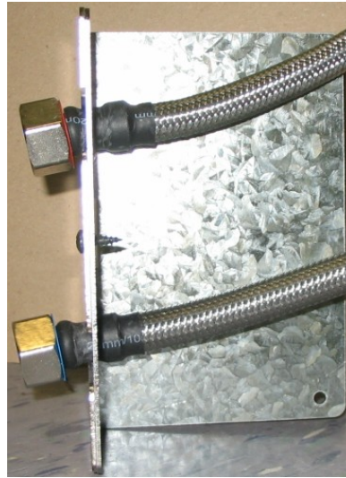
Step 8 assemble hose mount angle and hose clamp brackets
