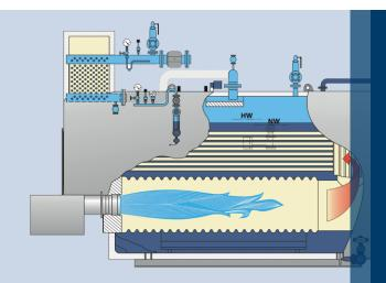
If superheated steam is required instead of saturated steam, a superheater module can be placed on the front reversing chamber. A bypass flap constantly controls the temperature of the superheated steam over a large load range. The smoke tube areas remain easily accessible thanks to the pivoting door of the reversing chamber.
