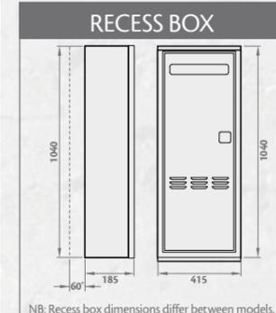
NB: Recess box dimensions differ between models.
