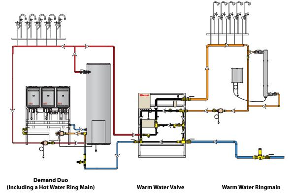
This is not a formal engineering drawing. Insulation not shown on site pipework. Ablution areas: temper as required. Installation as per local regulations. Details subject to change without notice. Non return and cold expansion valves are only required on circulating systems. Please refer to Rinnai Commercial Representative when designing systems. For ringmain pump selection consult Rinnai Commercial.
